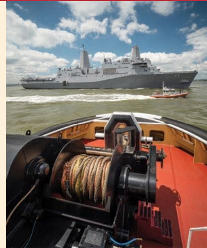
**The Markey DESF-48 bow winch, above, wrapped with 800 feet of 10-inch Samson line, awaits action as the tug approaches USS Arlington. Chief engineer Rob Smith, left, stands with one of the Caterpillar 3516E main engines. The diesels provide 80 metric tons of bollard pull.**
